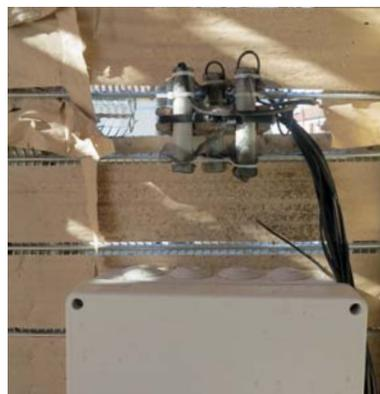
CAPTEURS HYGROTHERMIQUES ET CENTRALE D'ACQUISITION DES DONNÉES
